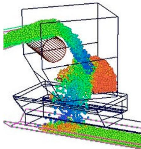
**Figure 4 Model of Rock Box Type Transfer**
