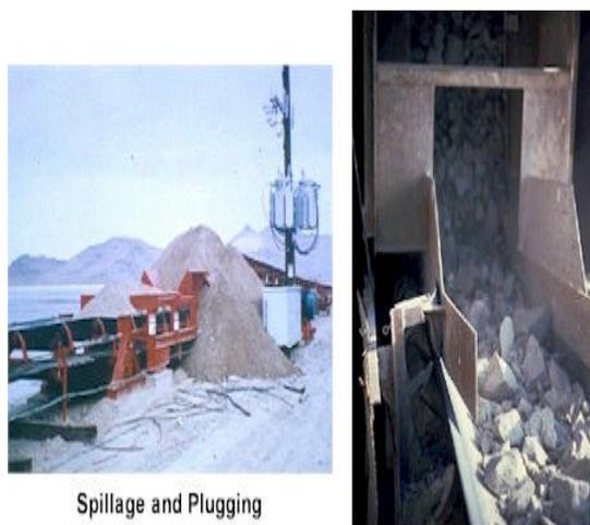
**Figure 1 Common Chute Problems**
