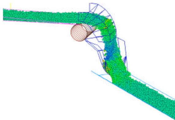
**Figure 2 Example of a Hood and Spoon Chute**
