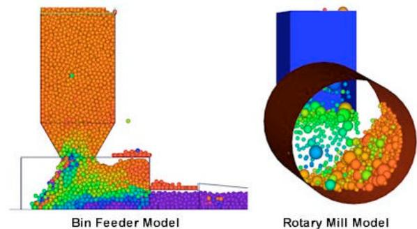
**Figure 3 Examples of the Application of DEM**
