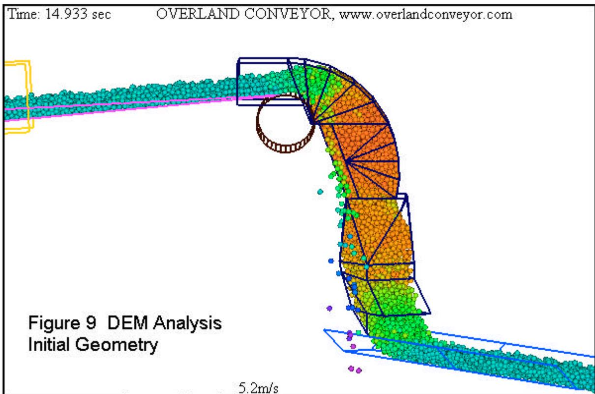
To date, the major area in which this method has been used in relation to conveyor systems has been in the design of transfer chutes. Traditionally, transfer chute design has been a black art, often with poor results. In fact it has remained one of the last intractable problems associated with conveyors. With the development of the Discrete Element Method, any chute geometry and a variety of material characteristics can be modeled and the resulting behaviour observed.
