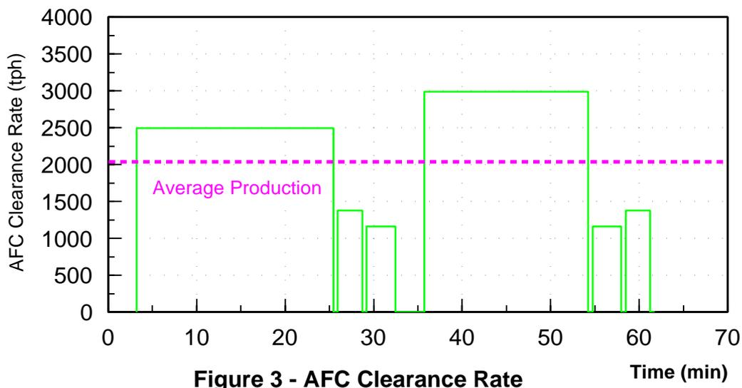
If a cutting cycle such as this is used, while the shearer needs to be sized at only 2750tph, the AFC and conveyors must be sized for 3000tph and the average production for a perfect cycle is only 2000tph.
