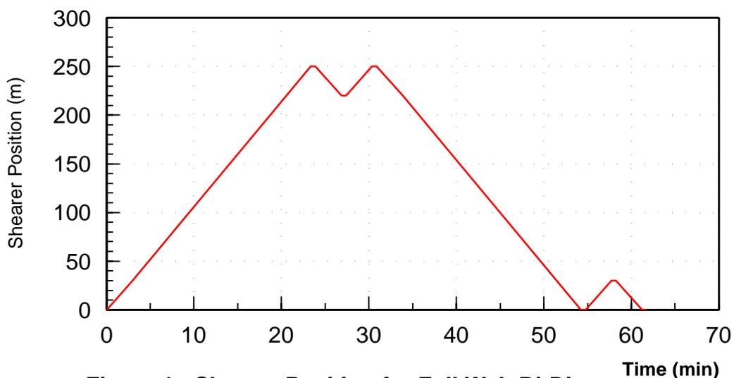
**Figure 1 - Shearer Position for Full Web Bi-Di**
