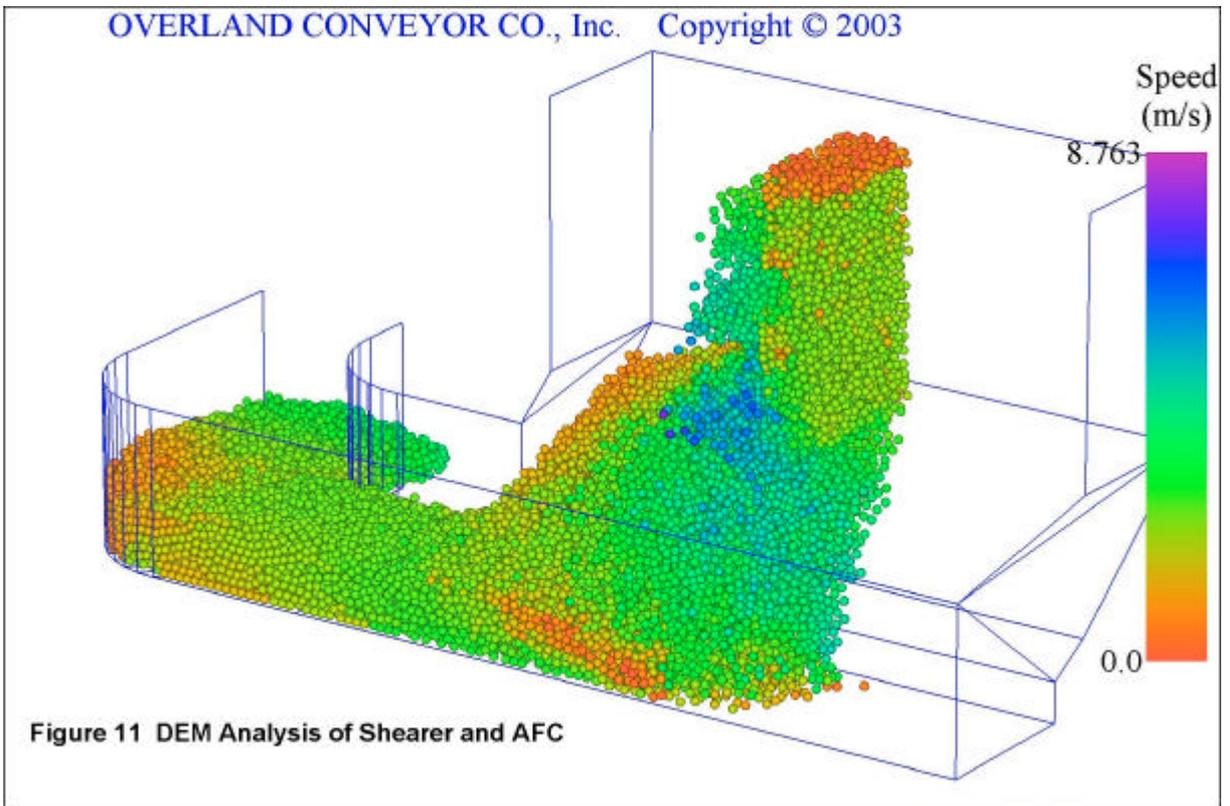
The latest research in this field is looking at modeling the actual longwall operation, including the Shearer and AFC. Currently little or no science is used in the design and analysis of these components. With the ability to visualise the mechanics of these elements in operation, it is expected that better designs will be forthcoming. Figure 11 shows a simple model of a shearer and AFC in operation.
